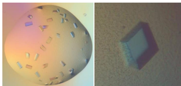
Images of HSP90 (N-term domain) crystallized in C3 for MecRx from SG1 (ShotGun) Screen (courtesy of J. Newman, CSIRO)
